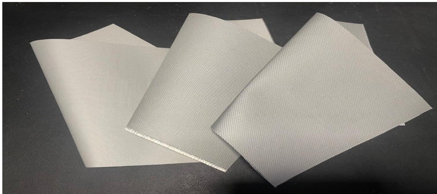
ABOVE RIGHT TO LEFT 30 minute rated—60 minute rated—90 minute rated as stated integrity only
